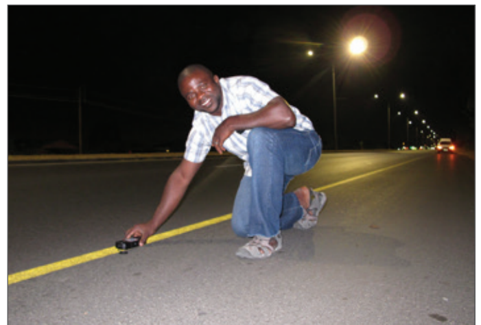
Figure 10: Brice Tsozbe validating light levels which had been installed as part of a street light energy saving project
