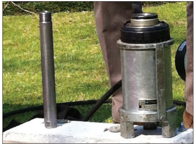
Figure 7: Preparing to conduct a pressure test on a friction anchor cast in concrete
